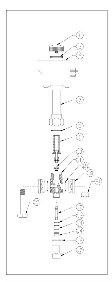
through the valve. When de-energized, the spring in the #9 Plunger-Needle-Assembly forces the valve closed.
