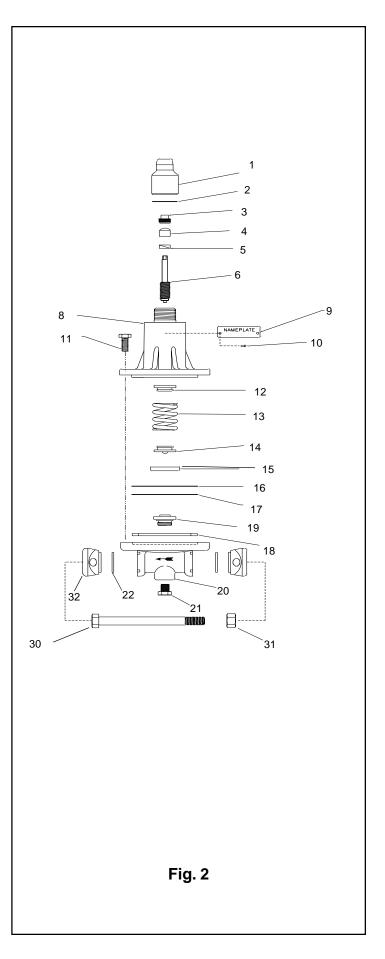
valve seat, thus reducing the flow. Once the inlet pressure drops below the regulator setting, the diaphragm closes off flow, subject to limits of the seat leakage tolerance, which is held to a minimum with the pilot seat design.
